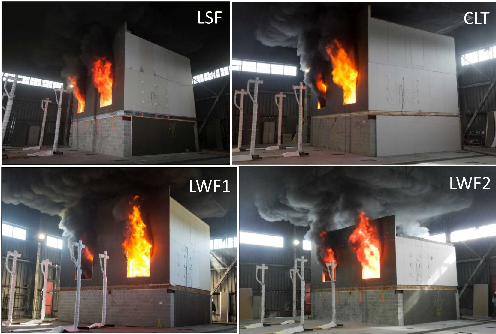
Figure 31. Flashover in both the bedroom and living room areas during large-scale apartment fire tests.
