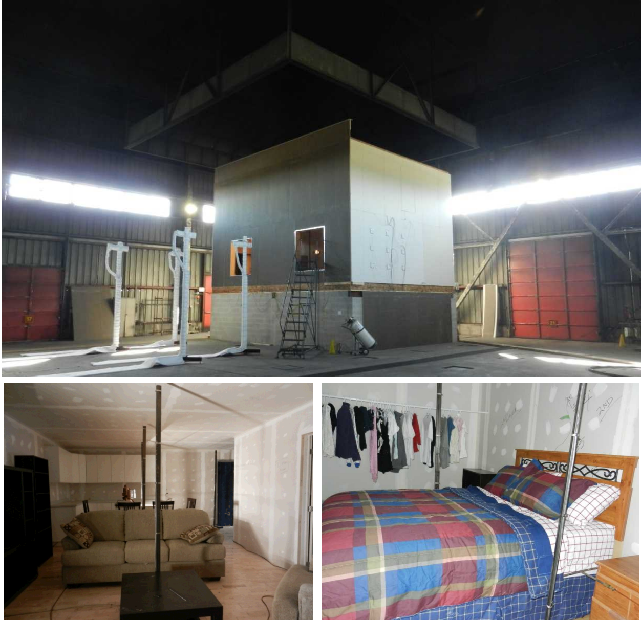
Figure 28. One of the large-scale apartment test setups.
