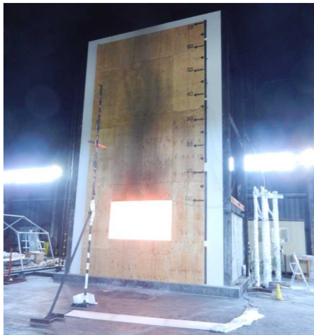
Figure 6. Tests of Exterior Wall Assemblies.
