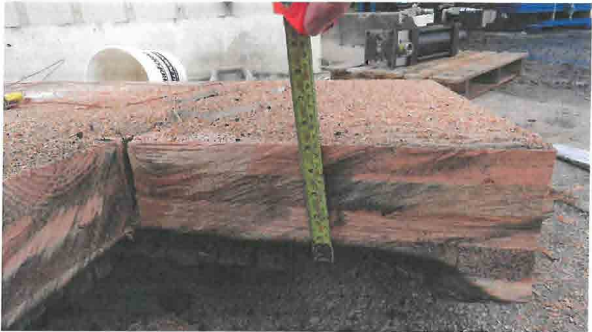
Figure E-7. Post Test Picture of the CLT Panel.
