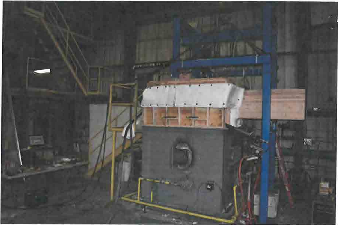
Figure A-5. Test Assembly Instrumented and Placed Inside Furnace.
