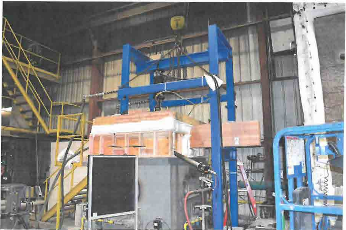
Figure A-6. Test Assembly Placed Inside Furnace.
