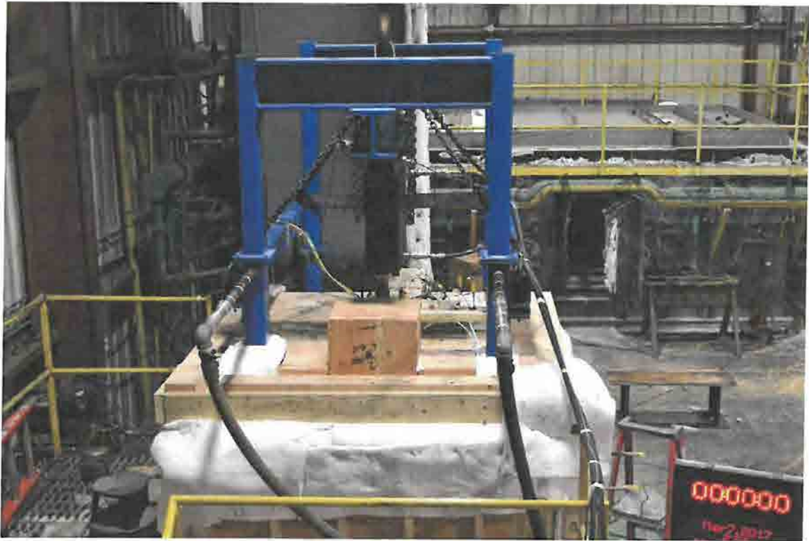
Figure E-1. View of the Assembly and Applied Load Equipment at Start of Test.
