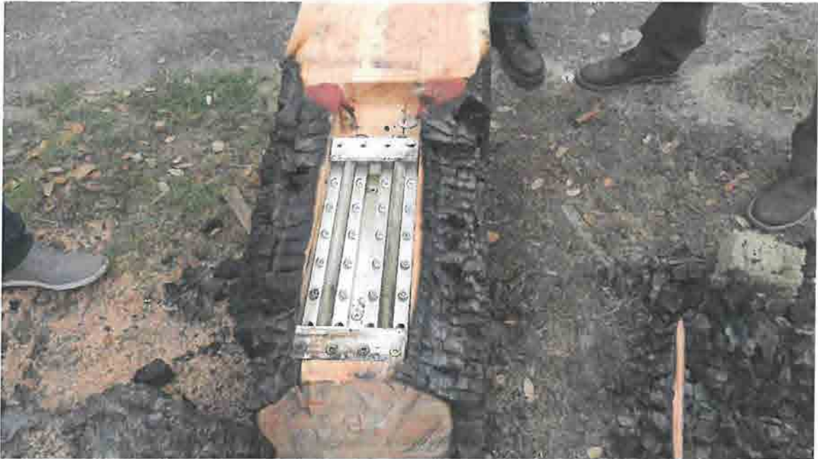
Figure E-7. Post Test Picture of the Steel Connection on Column (Misabeled B, Should be C).
