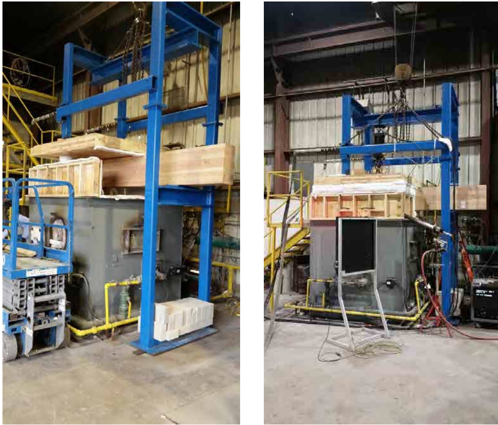
Figure 2 – Test specimen in loading frame with CLT floor attached to beam, within upright furnace
