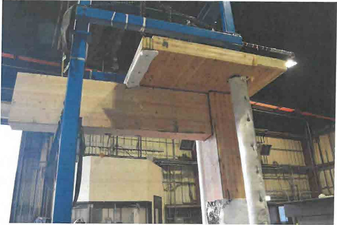
Figure A-5. Test Article Installed in Self-Reacting Frame.
