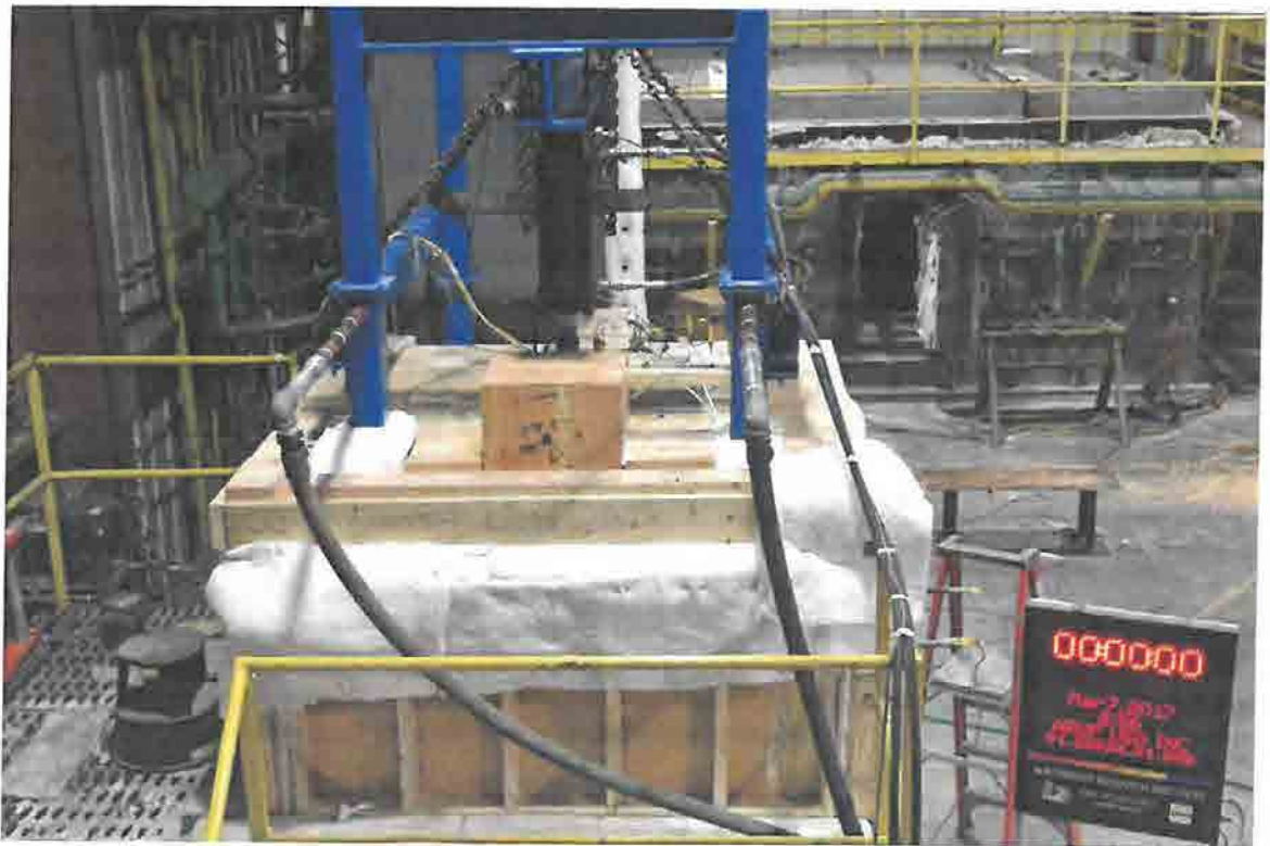
Figure A-6. Test Assembly Instrumented and Placed Inside Furnace.
