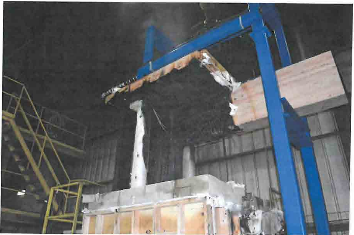
Figure E-4. View of Connection immediately after Test.
