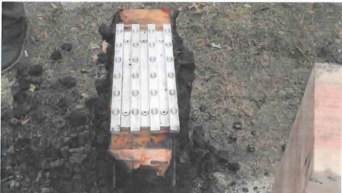
Figure E-8. Post Test Picture of the Steel Connection on Beam.
