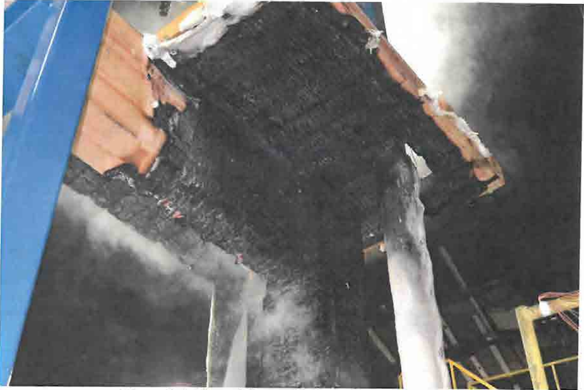
Figure E-5. View of Connection immediately after Test.
